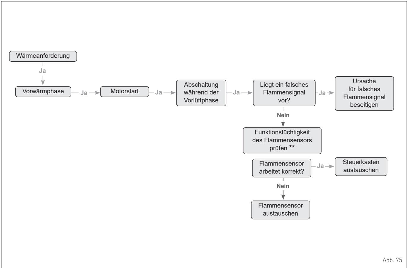
**(\*\*) FUNKTIONSKONTROLLE DES FLAMMSENSORS**
